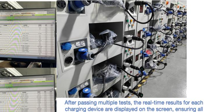
After passing multiple tests, the real-time results for each charging device are displayed on the screen, ensuring all equipment has met strict criteria, including continuity, insulation, and electrical safety.
