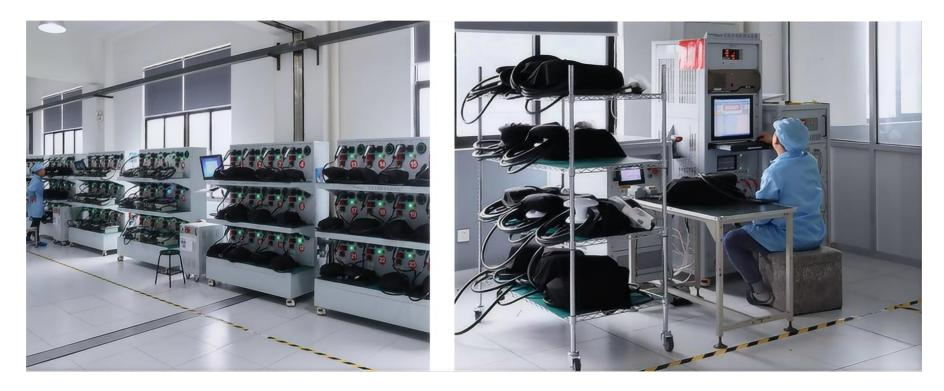
On dedicated testing workstations, all charging equipment undergoes rigorous electrical performance and durability tests. With advanced automated testing systems, we ensure that every device maintains the highest quality standards during mass production, avoiding any performance issues.
