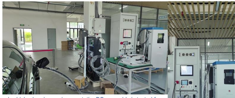
In a real vehicle charging environment, the DC gun cable is tested for stability and durability under various climate and load conditions.
