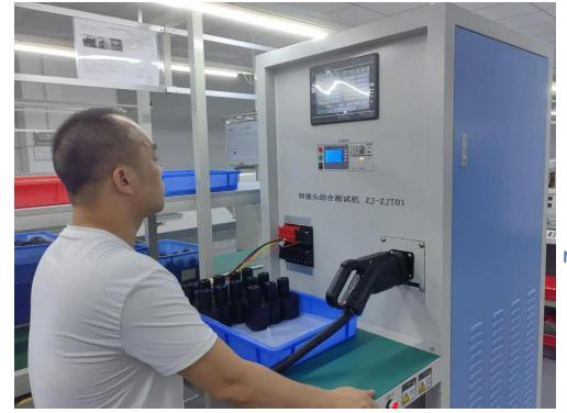
The electrical performance testing for DC charging connecter verifies their stability and safety under high-load conditions.
